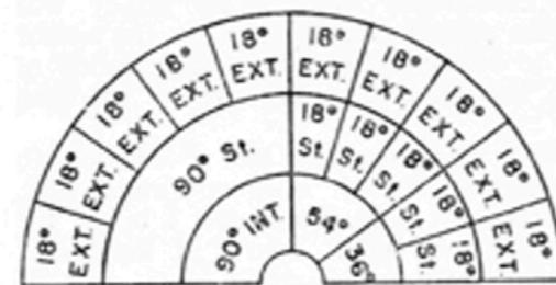
Track geometry (left) is based on classic "golden mean" with 90, 54, 36, 18 degree curves in differing sizes, plus straights, half straights, etc.
